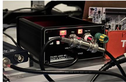
**Figure 4.3:** **Left:** Simplest yet functional circuit implementing the feedback controlled laser ablation protocol. The circuit implemented is more complex due to added safety features (see main text). **Right:** The physical circuit is encased in an aluminium box with BNC connectors and light indicators. A USB port at the front powers the device and allows for communication between the microcontroller and the computer.
